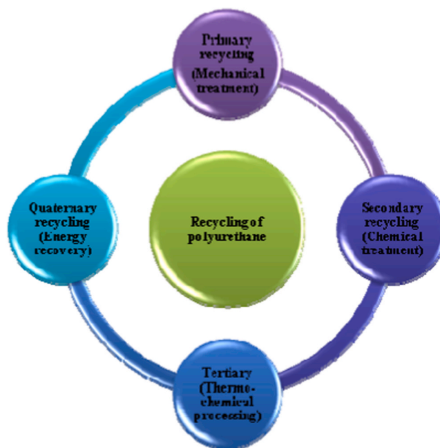
Fig. 6. Outline of polyurethane recycling.
