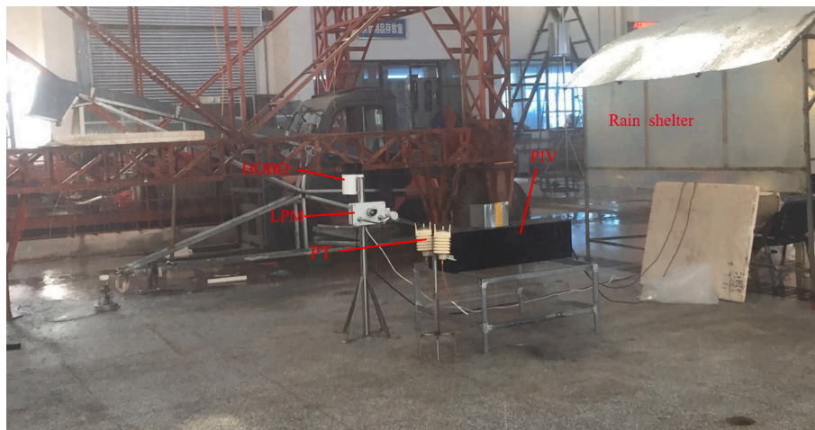
Fig. 4. General view of the experimental area and sensor setup under the rainfall simulator showing the three investigated sensors, tipping bucket rain gauge and recording rain shelter.
